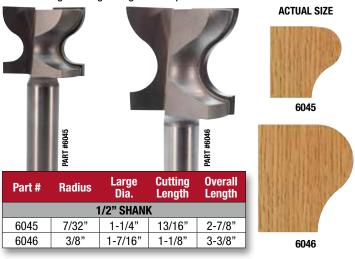
Use bearing (B16 for #6045, B18 for #6046) and Lock Collar (LC-1/2) on shank for template work.
