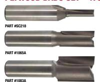
These router bits are sized to exactly match today's nominal plywood thicknesses. Consists of a 7/32" bit for 1/4" Plywood, a 31/64" bit for 1/2" Plywood, and a 23/32" bit for 3/4" Plywood. Included:
